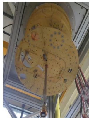
Paragraf GHS mounted on an Oxford Instrument’s Proteox development fridge
